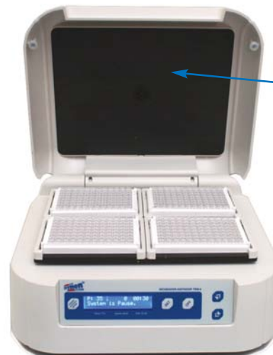
Cover inner plate with heating system.
